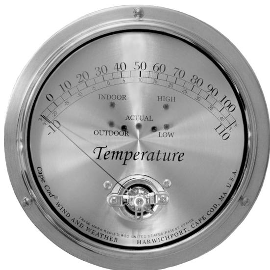
**INSTALLATION:** Using the included screw, attach the temperature Sensor outside on the North (preferably) side of the building, at least 3 feet above the ground, where it will not be exposed to direct sunlight or any heat sources such as louvers, vents, etc. Run the Sensor wire from outside to the indoor location of the dial. **Do not cut the wire:** the instrument is calibrated to use all 50 feet of wire. Keep any leftover wire coiled up and out of the way (e.g., inside the wall).
